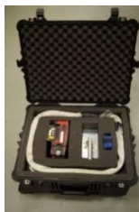
Fig. 4 - EMAT Heat Inspection complete equipment in its travelling case.
