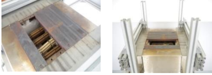
Fig. 5 - Left: various testing blocks on top of the heating box. Right: structure of aluminium profiles on the heating box.
