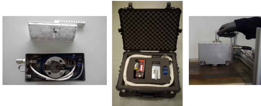
Fig. 44 - Left: scanner prototype inside view. Center: the equipment in its respective travelling case. Right: scanner prototype outside view.
