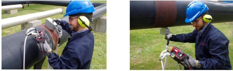
Fig. 71 - Left: EMAT Heat Inspection prototype on a OD 400 mm pipe. Right: Emat Heat Inspection prototype on upside-down test (same pipe as left image).
