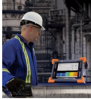
Fig. 26 - Eddyfi Lyft with Single Element PEC Probe being used at on-site inspections [70].
