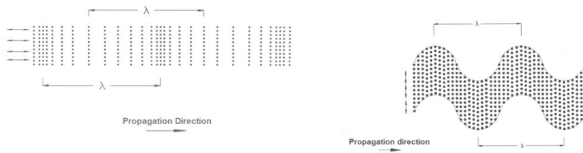
Fig. 8 - Left: Longitudinal wave. Right: Transversal wave (adapted from [34]; \lambda corresponds to the respective wavelengths).
