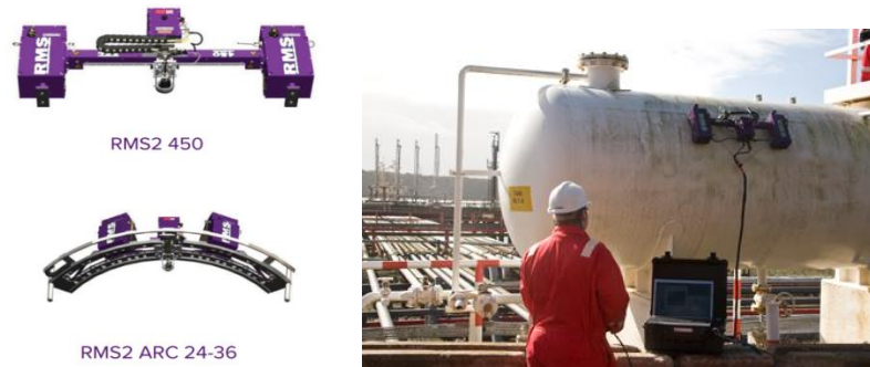
Fig. 20 - Left, up: RMS2 450 equipment. Left, down: RMS2 ARC 24-36 equipment [57]. Right: industrial application of RMS2 450 [58].
