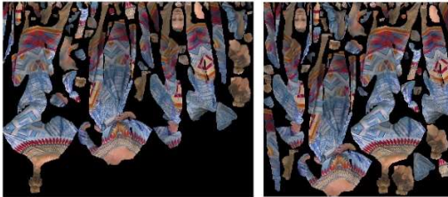
Figure 5 - Longdress PC packing: (left) V-PCC; (right) SPBP packing with HCBL+ES relative sorting metrics combination and Height absolute sorting metric for the first patch.
