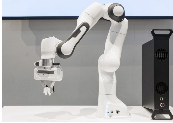
Figure 5.6: Panda robotic arm and respective control box (extracted from [26]).
