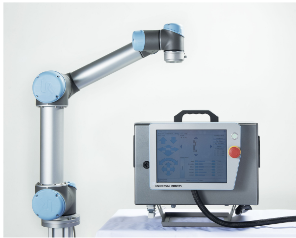
Figure 5.7: UR5 robotic arm, along its control box and teach pendant (extracted from [27]).
