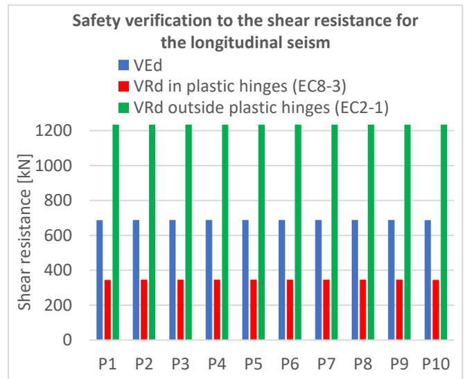
Figure 4.5. Safety verification to the shear resistance for the longitudinal seism
