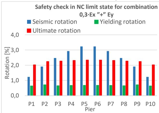
Figure 4.4. Rotation safety check in NC limit state for combination 0,3-Ex '+' Ey
