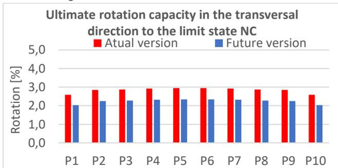
Figure 5.2. Ultimate rotation capacity of the piers in the transversal direction to the limit state NC
