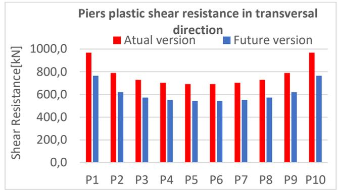
Figure 5.4. Piers plastic shear resistance in transversal direction
