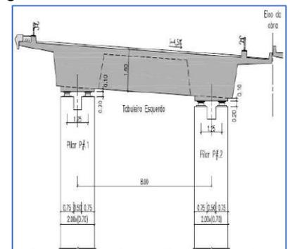
Figure 4.1. Cross section of the viaduct in the alignment of the piers
