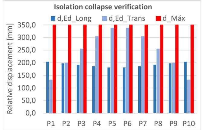
Figure 6.2 Isolation collapse verification.
