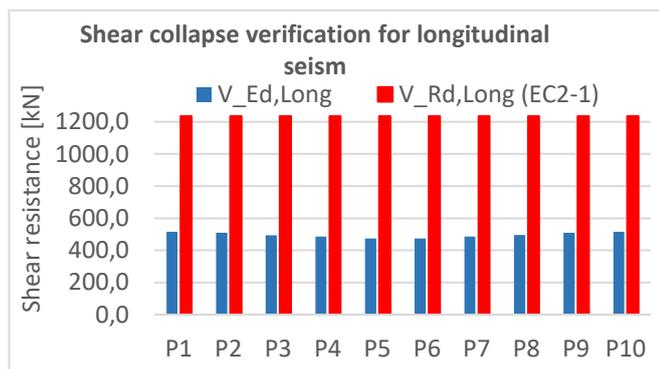
Figure 6.5. Longitudinal shear collapse verification
