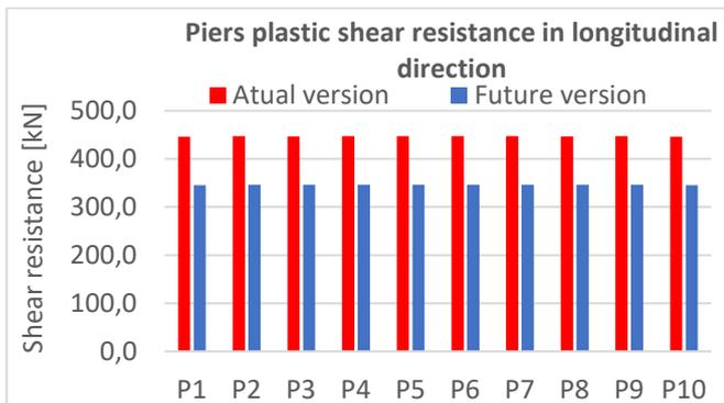
Figure 5.3. Piers plastic shear resistance in longitudinal direction
