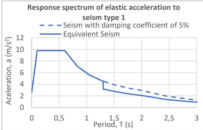
Figure 6.1. Response spectrum of elastic acceleration to seism 1
