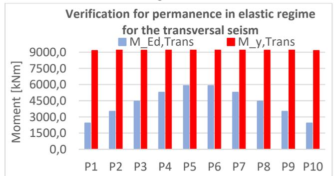
Figure 6.4. Verification for permanence in elastic regime for the transversal seism
