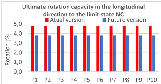
Figure 5.1. Ultimate rotation capacity of the piers in the longitudinal direction to the limit state NC
