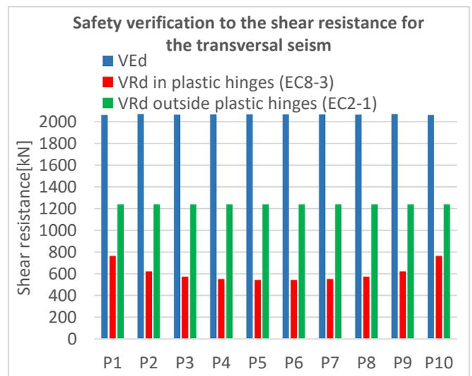
Figure 4.6. Safety verification to the shear resistance for the transversal seism
