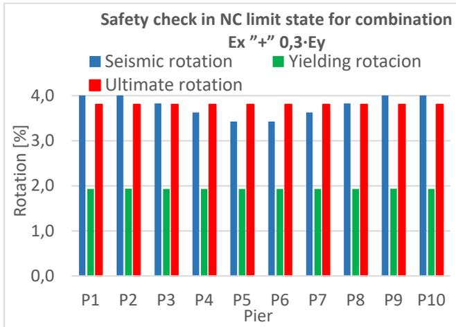
Figure 4.3. Rotation safety check in NC limit state for combination Ex '+' 0,3-Ey
