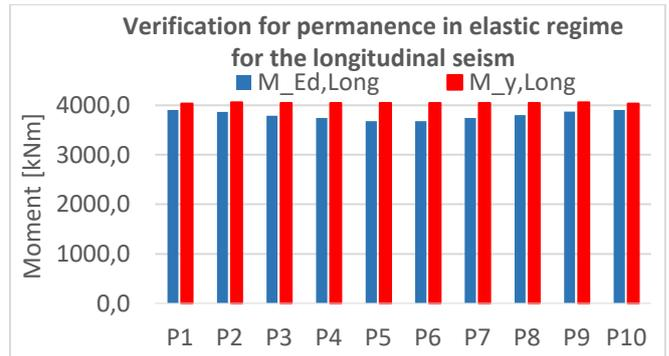
Figure 6.3. Verification for permanence in elastic regime for the longitudinal seism
