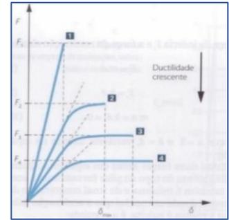
Figure 3.1. Force-displacement diagrams of a pillar to various ductility levels
