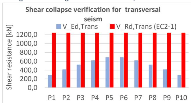
Figure 6.6. Transversal shear collapse verification
