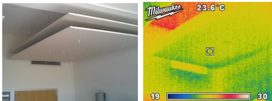
Figure 5- a) Real image of set PSb; Thermographic image of set PSb at 5:15 pm
