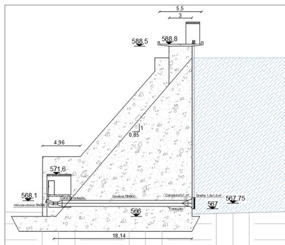
Figure 1 – Bottom outlet. Longitudinal section
