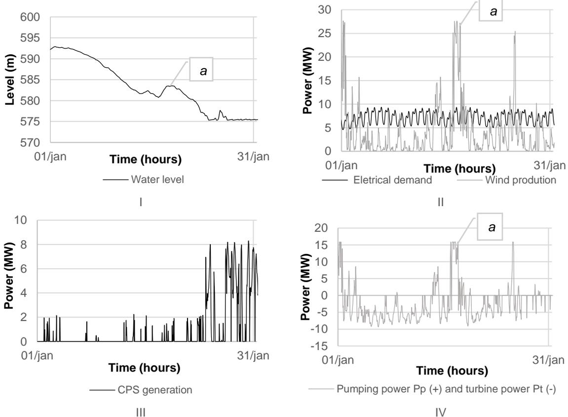
Graphic 3 – I) Water level variation in the reservoir II) Wind production and electrical demand III) CPS generation IV) Pumping and turbine power requirements (Case C3.2)
