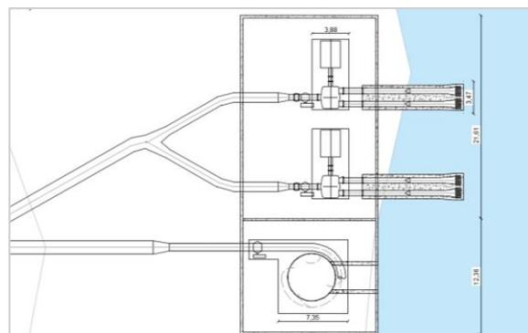
Figure 3 – Powerhouse with a Pelton turbine and the two pumps installed (Plant).
