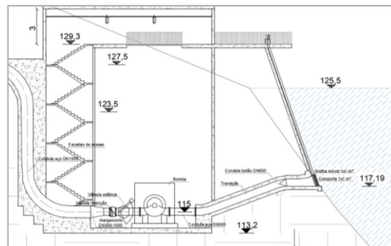
Figure 2 - Water intake of the powerhouse (Longitudinal section)
