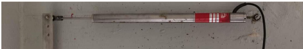
Figure 4: LVDT type DCRH2000C/371
