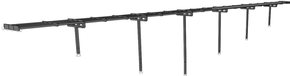
Figure 10: São João das Areias bridge numerical model
