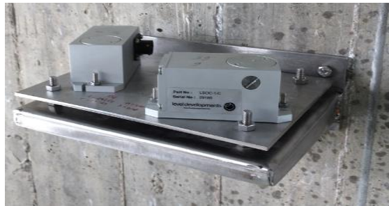
Figure 3: inclinometers of th type LSOC-1-C
