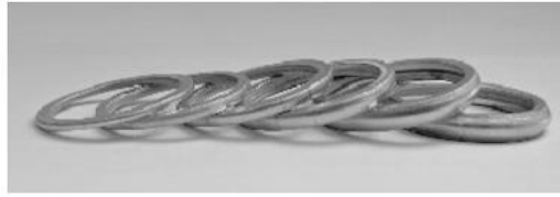
Fig. 6 - Upset compression of thin-walled rings between flat parallel platens.
