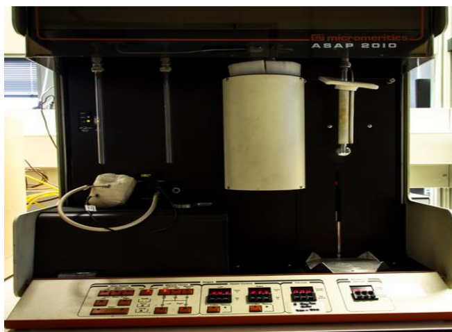
Figure 3.3 Micrometrics ASAP 2010 equipment available at Instituto Superior Técnico
