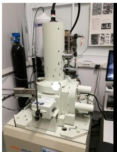
Figure 3.5 SEM: Analytical JEOL 7001F FEG-SEM available at MicroLab Electron Microscopy Laboratory (adapted from IST website)
