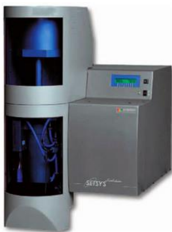
Figure 3.6 TGA-DSC Setsys Evo 16 device (Setaram) equipment available at Instituto Superior Técnico
