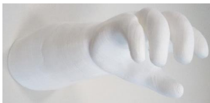
Figure 7: Final result after support removal and polish.
