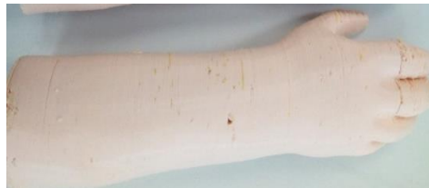
Figure 8: Final print result of NinjaFlex® -ABS print.
