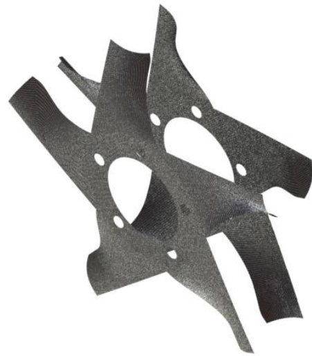
Fig. 14 - Ply reinforcement 3 present in the spokes
