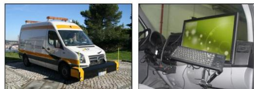
Figure 1 - Road Surface Tester Laser
