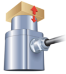
Figure 5: Schematic of a modified transient plane source method (MTPS)[W3]
