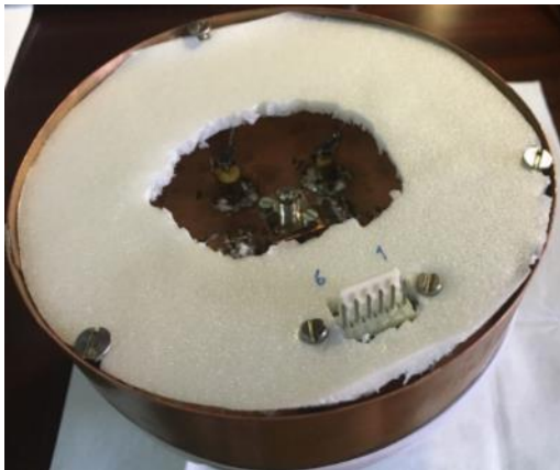
Fig. 12 - Fastened printed circuit board the styrofoam plate
