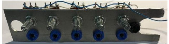
Fig. 13 – Control device parasitic monopoles
