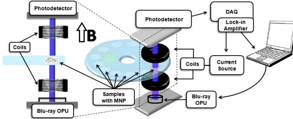
**Figure 1:** Schematic illustration of the optomagnetic readout set-up used in the approach described in this study.
