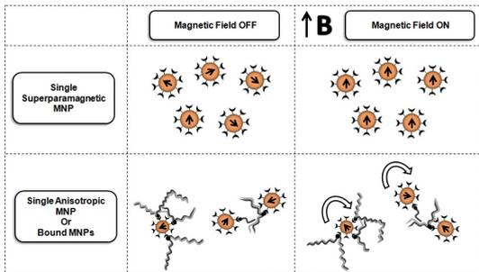
**Figure 2:** Representation of the response to a uniaxial magnetic field for single superparamagnetic MNPs, anisotropic MNPs with remnant moment and clusters of MNPs.
