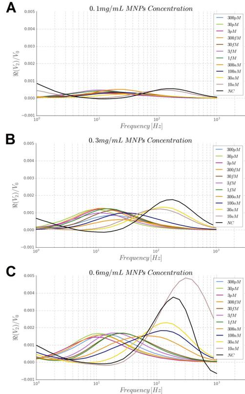
**Figure 4:** Comparison between optomagnetic signal for different MNPs concentrations for Dengue-2 synthetic target. LAMP was allowed to react for 30 minutes at 67° C. Three repetitions of each serial dilution concentration was done to provide statistics for the dose response. A - 0.1mg/ml MNP concentration. B - 0.3mg/ml MNP concentration. C - 0.6mg/ml MNP concentration.
