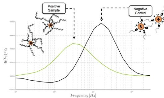
**Figure 3:** Representation of the difference in  $\Re(V_2)/V_0$  for solutions of MNPs with different hydrodynamic volumes.
