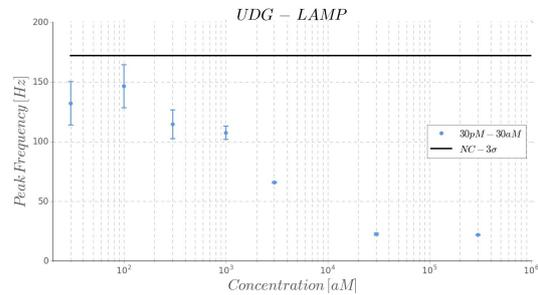
**Figure 7:** Frequency of the peaks with respect to concentration of target, with representation of the negative control in the  $NC - 3\sigma$  parameter. The error bars correspond to one STD from three repetitions experiments for each concentration.
