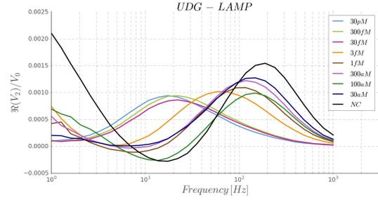
**Figure 6:** Average  $\Re(V_2)/V_0$  signal obtained from UDG-LAMP in the  $30\text{pM} - 30\text{aM}$  concentration range. The average signal was the result of three repetitions for each concentration.
