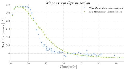
**Figure 9:** Optimization of magnesium concentration for RT-LAMP in terms of reaction velocity and noise in the signal.
