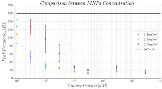
**Figure 5:** Peak frequency plots with respect to concentration for the different bead concentrations used. Blue, green and pink correspond to 0.1, 0.3 and 0.6mg/ml concentration. The error bars are the result of one STD calculated from triplet experiments.
