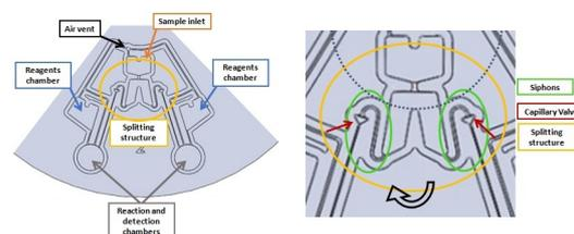
**Figure 14:** Schematic representation of the features of the first design for multiplex cartridge.
