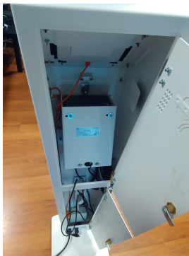
Fig. 12. Photo of the kiosk from the back, with opened doors, where we see the tablet attached to the frame, the printer compartment.
