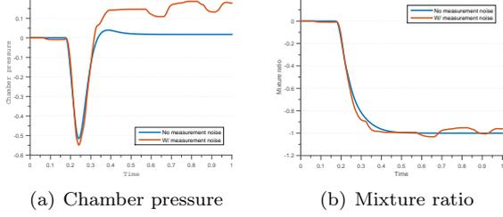
Figure 6: Output time response to a step of mixture ratio  $MR = -1$  on the complete linear model.
