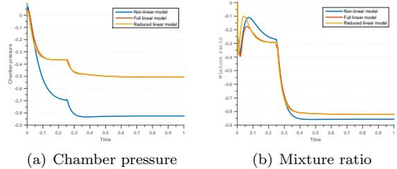
Figure 3: Linear and non-linear models time-response comparison to a VBPH and VBPO section steps of 1% of the nominal value.
