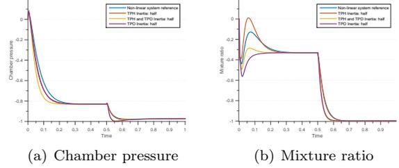
Figure 5: Step time-responses for varying moments of inertia of the turbo-pumps.
