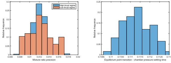
(a) Mixture ratio precision- required maximum: 0.033 (b) Chamber pressure settling time- reference value: 0.1096
