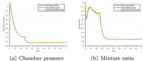
Figure 4: Linear and non-linear models time-response comparison to a VBPH and VBPO section steps of 1% of the nominal value.
