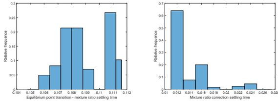
(c) Mixture ratio settling time- reference value: 0.1096 (d) Mixture ratio correction settling time- required maximum: 0.028
