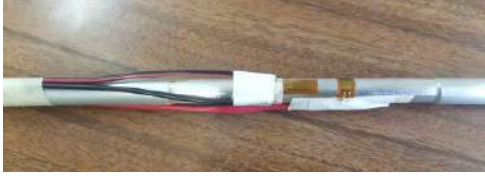
Figure 7: Strain gauges placed on the sensing bar.
