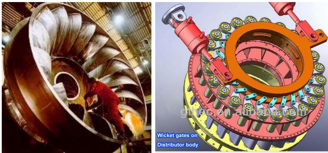
Figure 3-2: Details of a Francis turbine.
