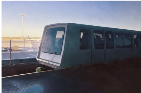
Figure 3.20: The Stansted Airport Transit System conveys passengers between Terminals 1 and 2 of Stansted Airport, United Kingdom (source: Wikimedia). Vehicles have no driver. They stop, open doors, close doors, and move between terminals automatically.
