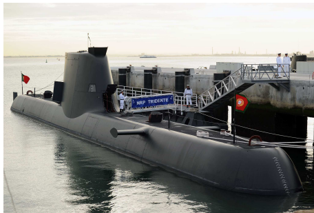
Figure 3.23: The Portuguese Navy submarine Tridente, of the Tridente class, propelled by a low noise skew back propeller and powered by hydrogen–oxygen fuel cells (source: Wikimedia).
