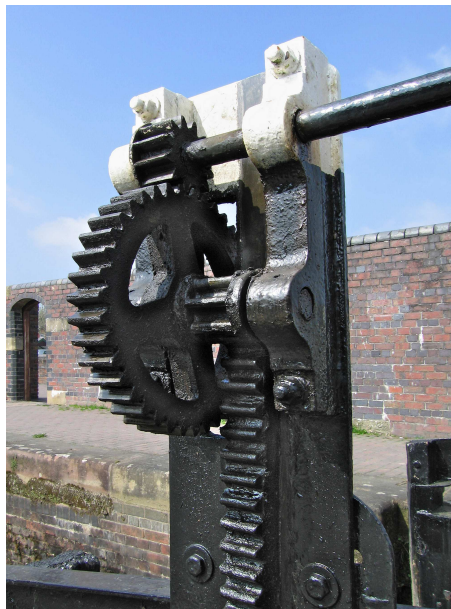
Figure 4.14: Left: rack and pinion in a canal gate; the rack is the linear element (in this case, vertical). Right: schematic of a harmonic drive. (Source: Wikimedia.)
