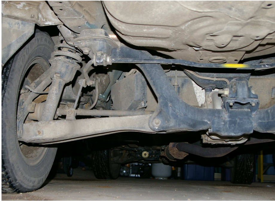
Figure 4.6: Independent suspension of a car's wheel (source: Wikimedia). The spring is clearly visible. The damper can be seen inside the coils of the spring.
