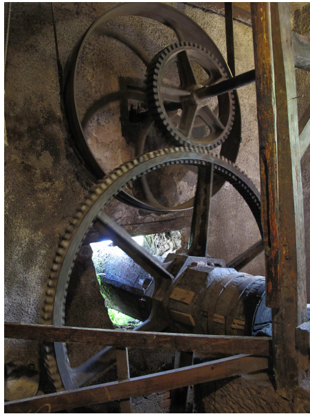
Figure 4.13: Left: two external cogwheels (source: Wikimedia). Right: two cogwheels, the outside one being an internal cogwheel (because the cogs are on the inside), and the inside one being an external cogwheel (because the cogs are on the outside; source: https://etc.usf.edu/clipart ).
