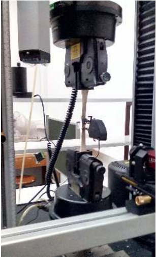
Figure 5.7: Parallel to grain test of the specimen.
