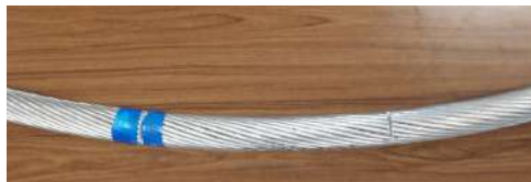
Figure 3.17: Cable with cuts two layers (right), and three layers (left) deep.
