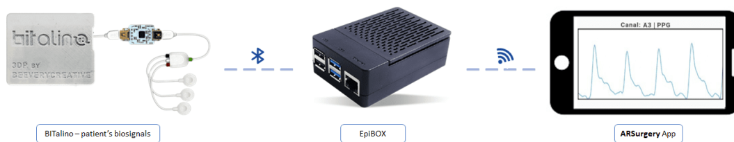
Figure 4.2: Architecture of the (optional) connection between ARSurgery and the BITalino measuring patient's biosignals, through the EpiBOX interface.
