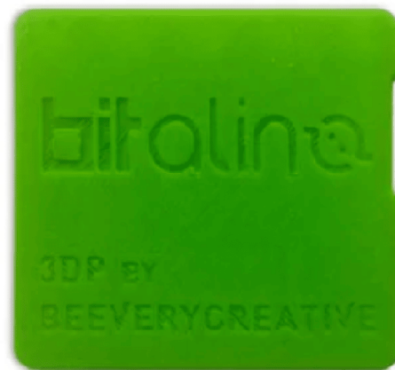
(b) BITalino (r)evolution Board BT/BLE protected with a 3D printed PLA enclosure
