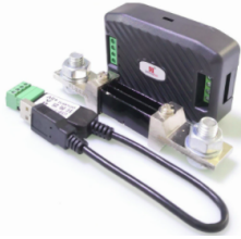
Figure 5.10: Photo of a similar PZEM current sensor to the one used in the vehicle.
