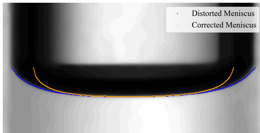
Figure 5.7: Detected meniscus interface in blue and the correction for the optical distortion of these points in orange
