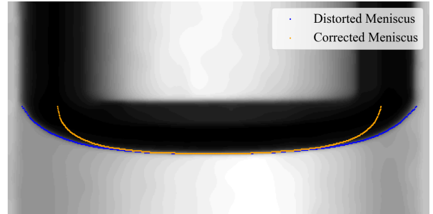
Figure 14: Figure with the detected meniscus interface in blue and the correction for the optical distortion of these points in orange
