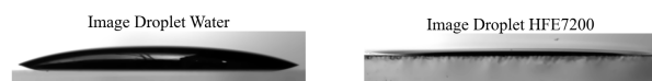
Figure 10: Captured image of a droplet of water and a droplet of HFE7200, where it is possible to see that the higher contact angle of water allows makes for a more clearly defined droplet
