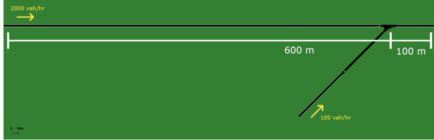
Figure 5.1: Network configuration of the first preliminary experiment: single-lane highway with merge section
