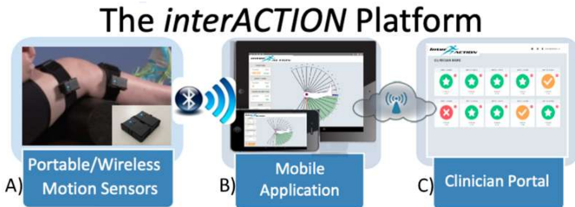
Figure 3.1: interACTION platform components: (A) wireless motion sensors attached to the knee of a patient; (B) screenshots from the current version of the mobile app; (C) screenshot from the current version of the clinician portal. iA provides real-time exercise feedback to the patient and logs performance metrics for remote clinicians to allow home exercise program monitoring. Image taken from [28].
