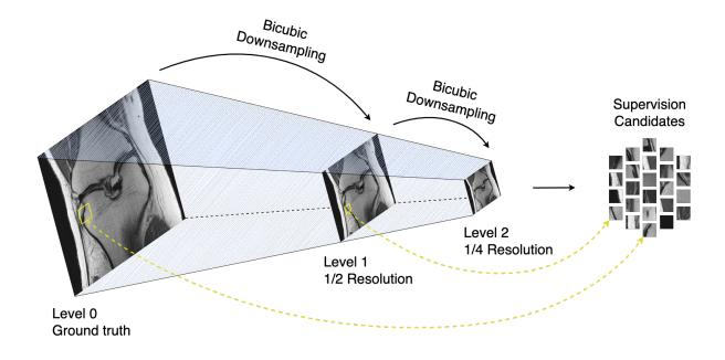
Figure 3.8: Beby-GAN 3-level image pyramid obtained with bicubic downsampling. Subsequent images are subject to repeated downsampling. Additionally, other types of degradation can be introduced in each subsampling level.
