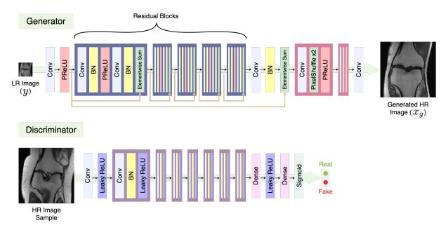
Figure 3.1: Basic architecture of SRResNet (SRGAN). Figure adapted from [13].
