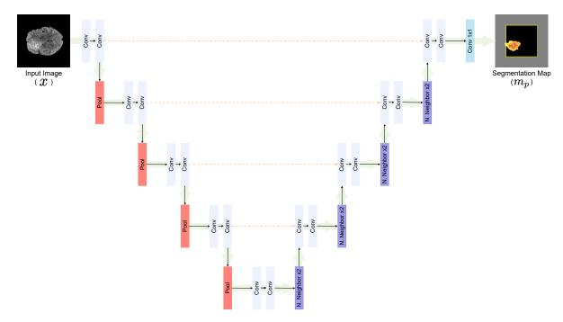
**Figure 5.6:** U-Net Architecture. Activation functions are omitted for visualization purposes and ease of comprehension. Feature map shape variations after every downsample and upsample step were not showcased for the same reason. Dashed orange lines denote skip connection and concatenation operations.
