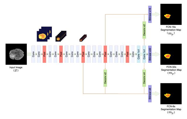
Figure 5.5: Architecture of FCN-32s, FCN-16s and FCN-8s. Feature maps are illustrated in a distinct colormap (not grayscale) for visualization purposes and ease of comprehension. Activation functions are omitted for the same reason.
