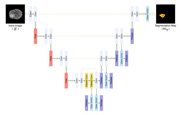
Figure 5.8: Open BraTS Solution Architecture. Dashed orange lines denote skip connection and concatenation operations.
