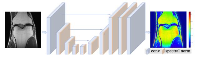
Figure 3.12: U-Net discriminator architecture with Spectral Normalization. Figure adapted from [63].
