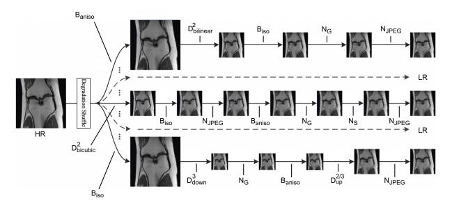
**Figure 3.7:** Proposed BSRGAN degradation model for a scale factor of 2. For scale a factor of 4, an additional bilinear or bicubic downscaling is applied. The type of blur employed is denoted by  $B_{type}$  and  $N_{type}$  is the type of noise. Meanwhile,  $D_{type}^{scale}$  stands for the downsampling applied under a defined scale. Figure adapted from [60].
