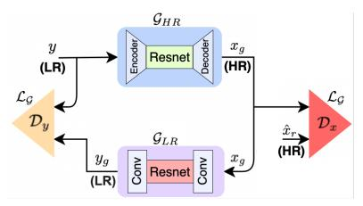
Figure 3.5: SRResCycGAN structure. Figure adapted from [57].
