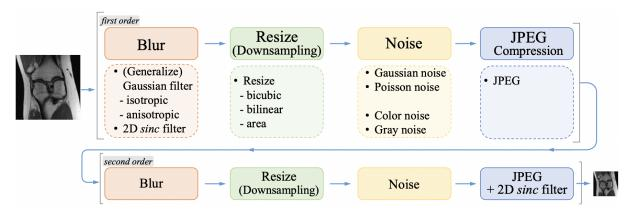
Figure 3.11: High-order Degradation Model. Figure adapted from [63].
