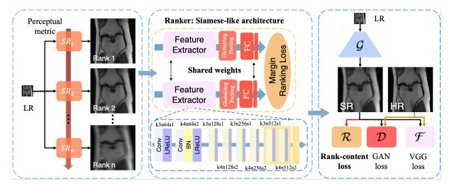
**Figure 3.4:** Overview of RankSRGAN. Essentially, RankSRGAN consists of a generator ( $\mathcal{G}$ ), a discriminator ( $\mathcal{D}$ ), a fixed feature extractor ( $\mathcal{F}$ ) and a ranker ( $\mathcal{R}$ ). Figure adapted from [54].
