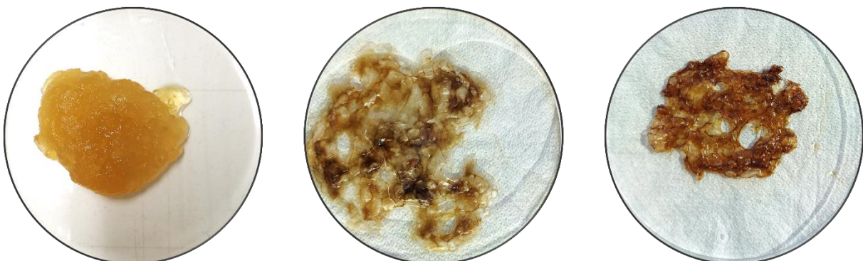
Figure 25. Left: extracted pectin before drying. Middle: extracted pectin with HCl (aq), after drying. Right: extracted pectin with 13% citric acid (aq), after drying.
