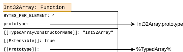
Figure 4.22: Representation of the Int32Array object.
