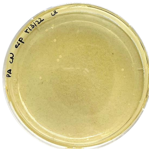
Figure 6. Example of a "neutralization method validation" plaque with E. coli ATCC 10536 for Suma Bac D10® after 24 hours of incubation at 37 °C.
