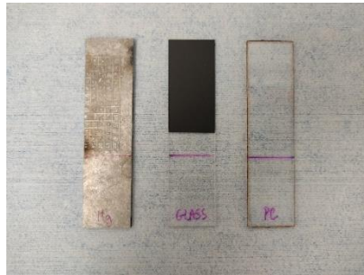
Figure 12 - Substrates employed in this study: magnesium alloy, painted glass and polycarbonate
