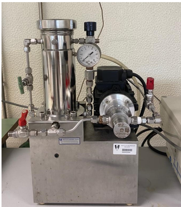
(a) CELFA P-28 ultrafiltration installation.
