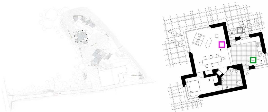
Figure 34 - Site plan and layout with location of measuring instruments (1–living room; 2–kitchen; 3–bedroom; 4–bathroom; 5–outdoor porch (source of site plan: EMBAIXADA, 2022)
