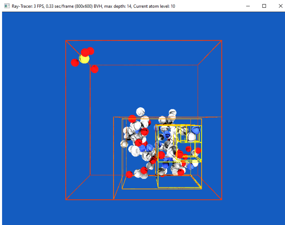
Figure 3.3: Visualization of a protein with 100 atoms, including the bounding boxes of nodes using BVH CPU.
