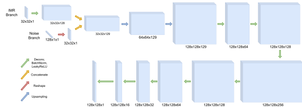
Figure 5: Structure of the Generator.
