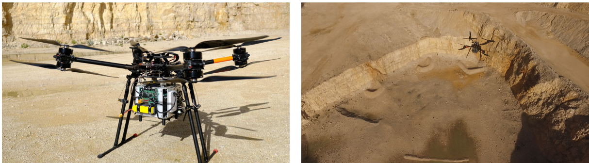
Figure 4.1: Spin.Works UAV from one landing mission on a quarry. On the left, we see the UAV with a monocular camera mounted underneath the electronic systems, pointing to the ground. On the right, we see it flying over a surface that looks similar to Mars, using a vision-based navigation system. The geometry of the problem is depicted on Figure 2.12. The images taken during this mission were extensively used during the performance evaluations made in this thesis. The dataset is described in section 4.2.2
