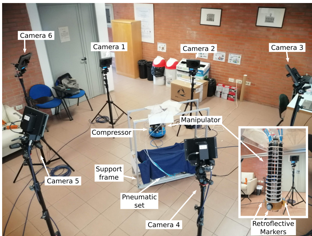
Figure 2.11: SMART-DX motion system used during the experimental tests
