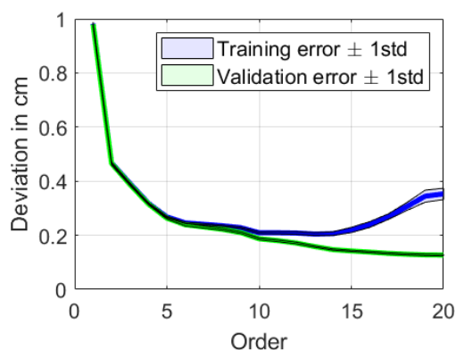
(a) Error of the direct kinematic model during the training and validation.
