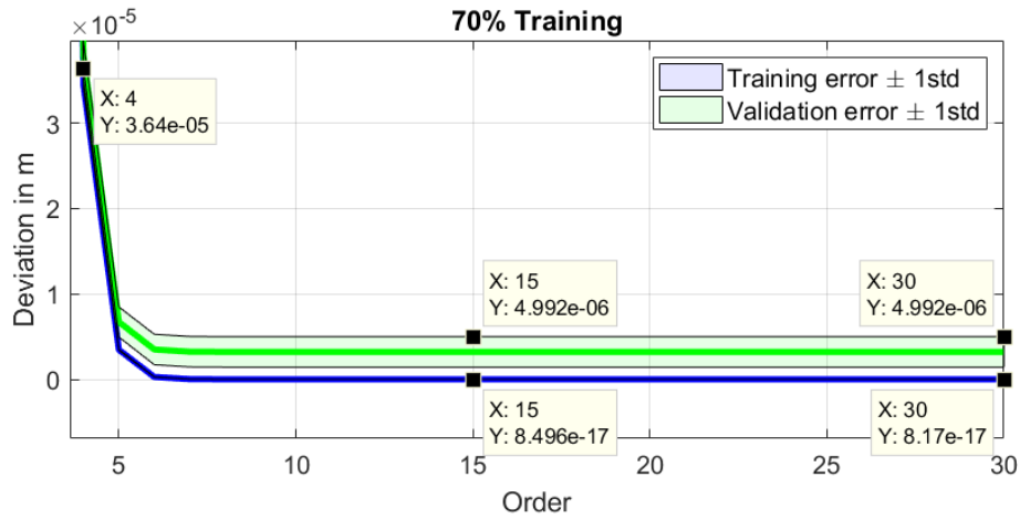
Figure 4.1: Direct kinematics model errors of BHA permutation data without noise with one cluster
