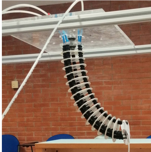
Figure 3.1: Proposed robotic arm in a bending configuration
