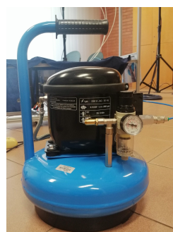
Figure 2.10: Compressor used as air supplier
