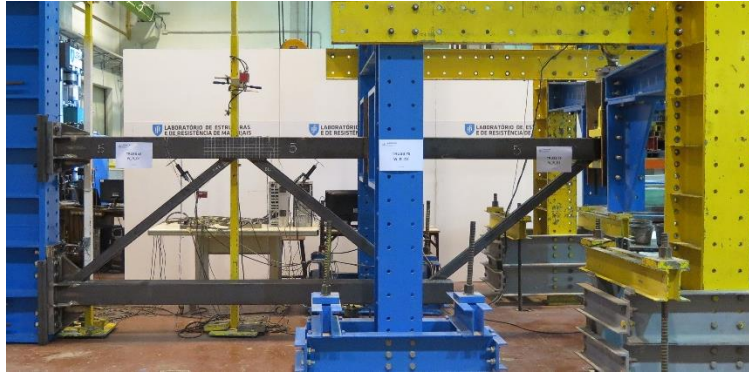
Figure 2.13: Experimental test on a Warren truss.
