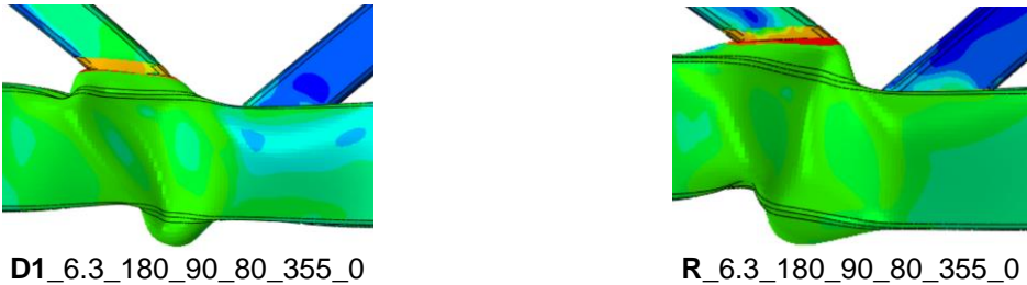
Figure 4.4: Critical joint deformation for t_0 = 6.3 mm.
