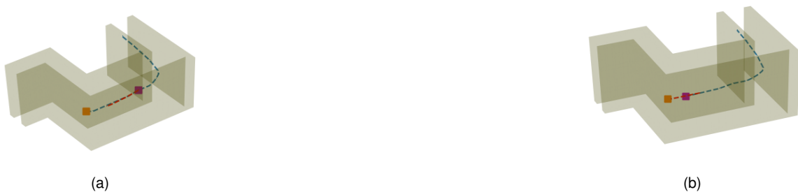
Figure 3.37: (a) an intruder is approaching at a high perceived velocity resulting in a potential collision. (b) In the time the intruder reaches the collision point, the quadrotor is not able to generate and escaping trajectory.
