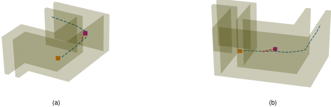
Figure 3.34: (a) Estimated future motion of intruder. (b) Potential collision detected.
