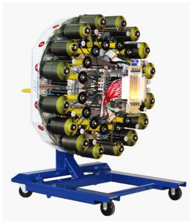
Figure 9 - Electroimpact's AFP head in a transfer cart [55]
