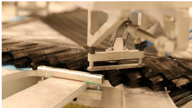
Figure 10 - Fibre tow being placed by a DFP machine (Provided by TU Chemnitz)
