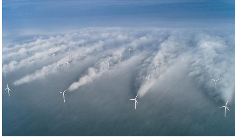
Figure 1.2.1 Wakes at Horns Rev wind park made visible by weather conditions [10]
