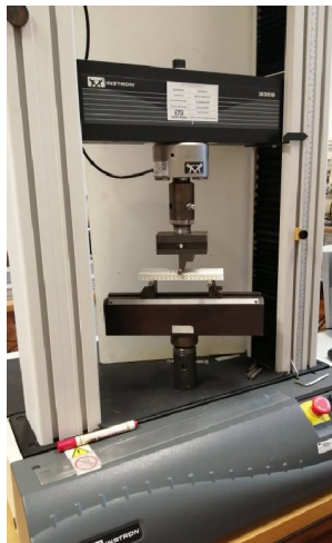
Figure 16: Instron 3369 - the equipment used for all the 3PB tests
