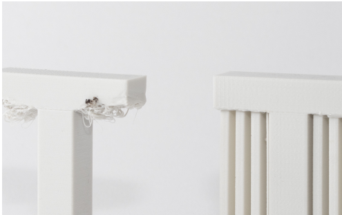
Figure 2.17: Failure caused by printing the letter T without support [33]
