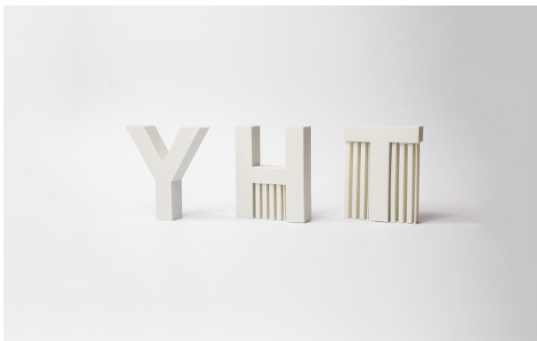
Figure 2.15: Overhangs and bridges represented by the letters Y, H and T [33]
