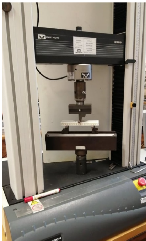
Figure 3.17: Instron 3369 with a specimen prior to initiating a procedure
