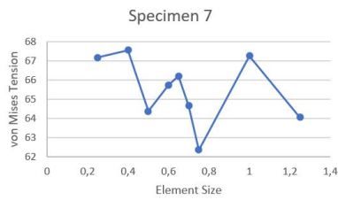
Figure 3.36: Mesh refinement for the specimen 7
