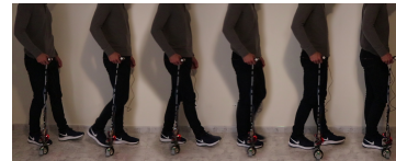
Figure 15: Test of the ability of the cane to keep up with the normal movement of the user.
