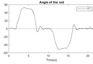
Figure 20: System response to the test of the cane’s ability to hold its position and support the user in the event of an imminent fall.
