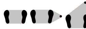
Figure 23: Support polygons in no cane (left), cane at side (middle) and cane at front (right) situations.
