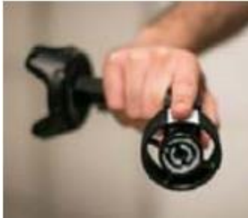
Figure 8 - Haptic Revolver in contact with the user finger 6
