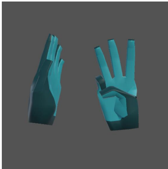
Figure 57 - Hand Figure for the Activation of Translation Mode using 2-Hands Interaction Model
