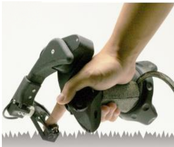
Figure 7 - Hand holding the Haptic device CLAW 5
