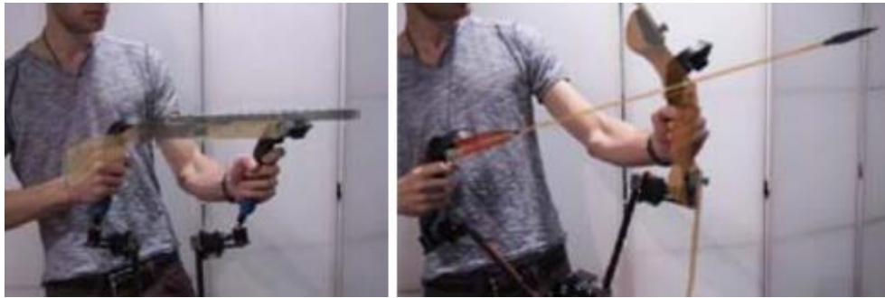
Figure 10 - Player using Controllers connected by Haptic Links and how it is perceived in the virtual environment (Gun on the Left, Bow on the Right) 7
