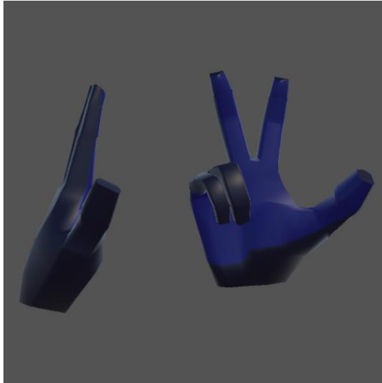
Figure 58 - Hand Figure for the Activation of Rotation Mode using 2-Hands Interaction Model
