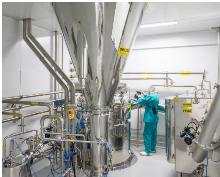
Figura 9- Representação de um spray dryer presente na Hovione (Retirada de https://www.hovione.com/products-and-services/contract-manufacturing-services/particle-engineering/technologies/spray-drying a 16/8/2020)
